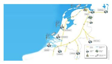
A national hydrogen backbone is being developed in the Netherlands, which will consist of 1,400 km of pipeline by 2030. The network will connect regional backbones with each other, with large clusters of industrial consumers and port facilities, as well as with storage facilities and grids outside the Netherlands. 85% of the backbone is expected to consist of reused gas infrastructure.
