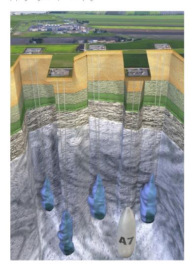
Dutch gas grid operator Gasunie is planning to develop its first large-scale hydrogen storage site at HyStock, Zuidwending. Here its subsidiary Energystock operates a storage facility with six underground salt caverns, which are currently used for storing natural gas. Four new caverns will be developed for hydrogen, with a total storage capacity of 20,000 tonnes.
