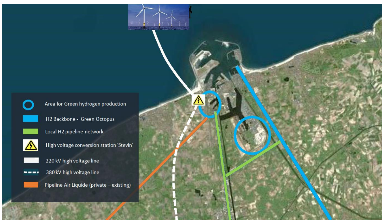
Figure 20: Possible configuration for a local hydrogen pipeline in the port of Zeebrugge in relation with a future hydrogen backbone
